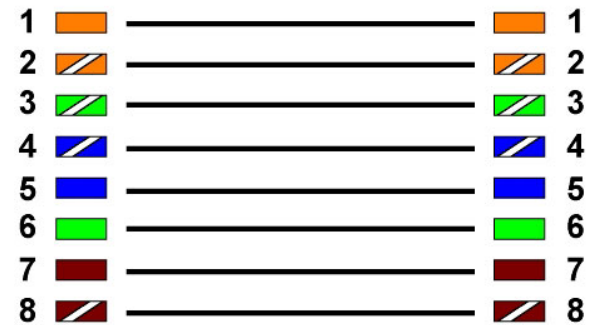
EIA/TIA T568B Straight Through Diagram
